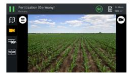
ISOBUS TC has an integrated camera view. The rear camera view can be configured to be automatically shown when reversing.
